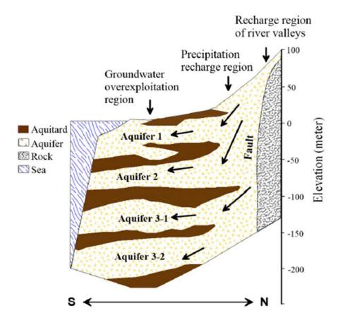
Figure 2. Hydrogeological profile of the Pingtung Plain.
